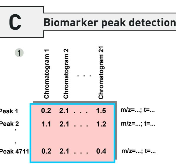
Importing the data matrix for multivariate analysis. Refined data arranged into a matrix of extracted peaks (rows) versus sample chromatograms (columns). Each matrix element corresponds to an individual peak volume (denoted by Expression Value in fig. 2).
